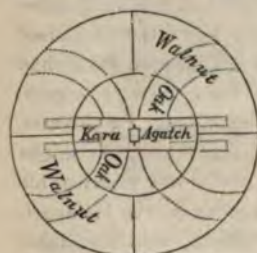
Section of Wheel of Armenian Cart.
