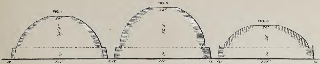
Figs. 1, 2, 3. Comparative sections of the large, or No. 1 Stūpa; as represented by different writers on Sānchi.
