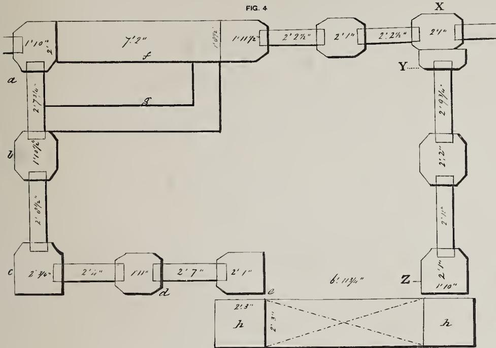
Fig. 4. Ground plan of the Northern entrance to the large, or No. 1 Stūpa (h h are the sculptured Gate-pillars).
